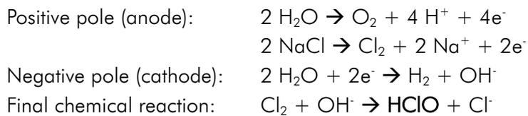
The operation requires a certain concentration of salt (4000 ppm), low enough that it normally will not be tasted. The **SSCmini**<sup>®</sup> automatically sanitizes your pool by converting the salt into Hypochlorous acid which kills bacteria and algae in the pool through a process called electrolysis.
