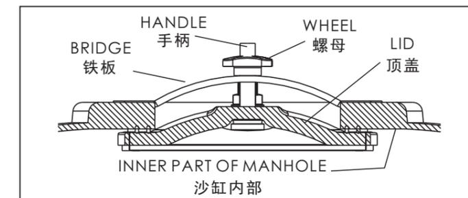
Introduce the lid in the manhole, leaving it leveled and centered. The lid must be supported by the handle, as this will avoid that it could fall into the tank and damage any of its parts. Put the bridge in the position shown and tighten manually the wheel. To achieve a proper seal, you do not have to tighten excessively the wheel, as this could damage the lid. The pressure itself will improve the seal.
